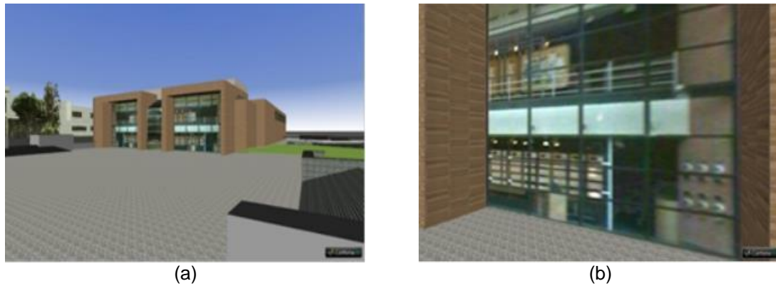
Figure 1. Pixelization in a 3D model of a campus [17]: (a) when viewed afar, (b) when viewed at close range
