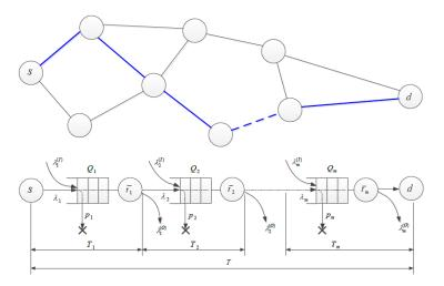
Figure 1. Routing model as a multi-phase queuing system
