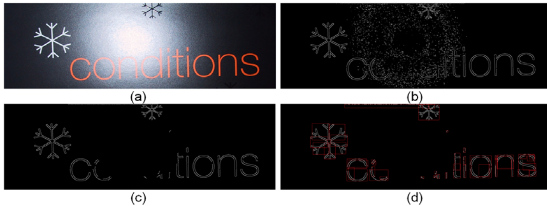
Figure 4. (a) Original Image; (b) Image after applying Canny edge detector; (c) Image after edge group filtering; (d) Initial edge pixel group
