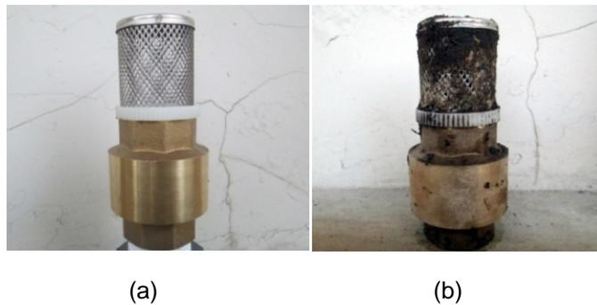
Figure 4. Foot valve examples; (a) A good foot valve;
