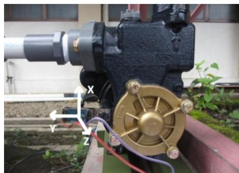
Figure 5. Attachment of the accelerometer on the water pump.
