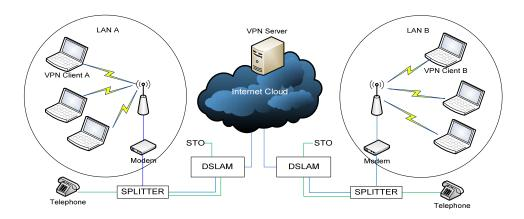
Figure 1. A topology of testbed network
