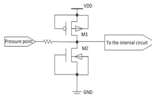
Figure 4. ESD protective circuit
