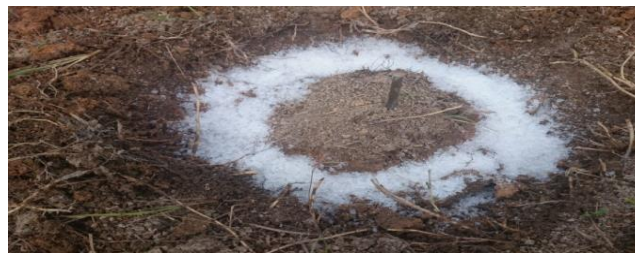
Figure 7. Salt is put around the electrode rod
