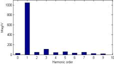
Figure 5. Harmonic contents of induced voltage for 4-pole winding
