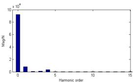
Figure 9. Harmonic contents of radial electromagnetic force
