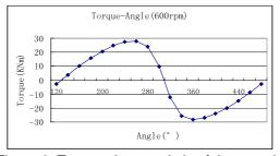
Figure 6. Torque characteristic of the sample DEBG
