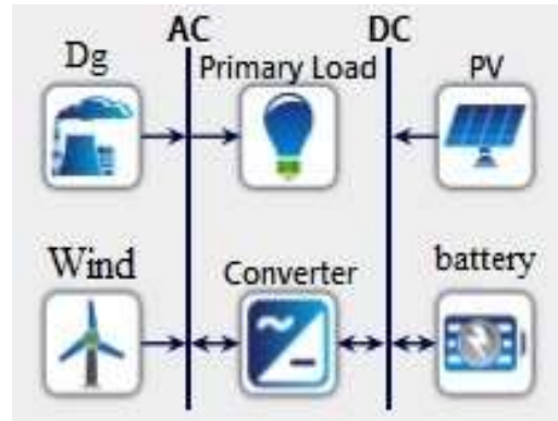
Figure 2. Hybrid model (off-grid) in HOMER
