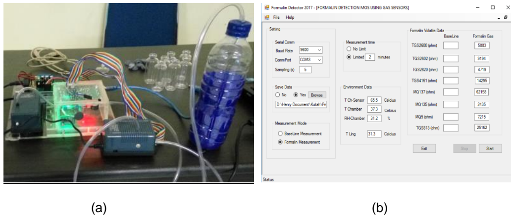
Figure 4. (a) Prototype and (b) acquisition software of the formalin vapor measurement.
