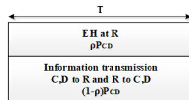
Figure 2. The energy harvesting and information processing in the proposed system
