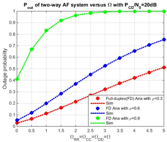
Figure 7. Outage probability versus  $\Omega$
