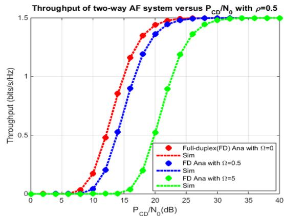
Figure 4. Throughput versus PCD/N0
