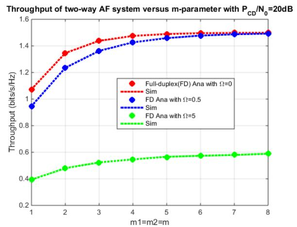
Figure 10. Throughput versus  $m=m_1=m_2$
