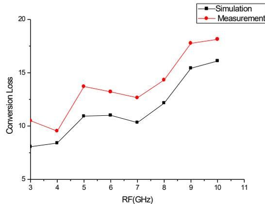
Figure 10. Simulated and measured conversion loss vs. RF
