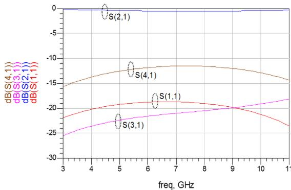
Figure 4. S-parameters of the single section coupled-line balun
