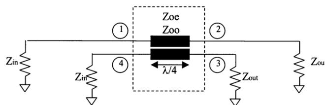
Figure 2. Four-port network for even- and odd mode [14]
