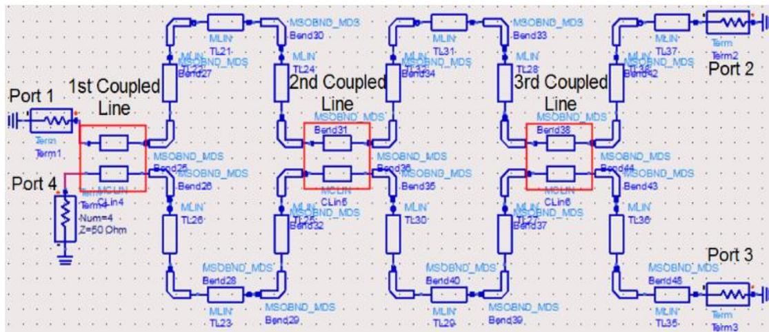
Figure 3. Schematic diagram of multi-section coupled-line balun
