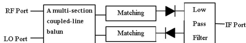
Figure 8. A multi-section coupled-line balun in the circuit of single-balanced diode mixer
