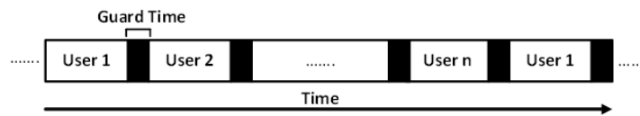
Figure 5. Illustration of TDMA time slot
