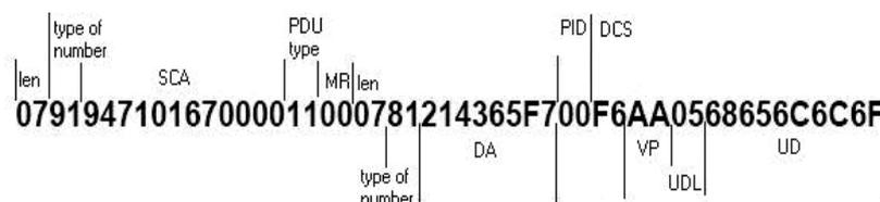
Gambar 1. Format PDU mode sms deliver (*mobile terminated*)
