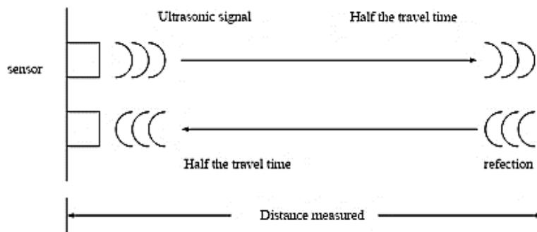
Figure 2. How ultrasonic sensors work [22-24]
