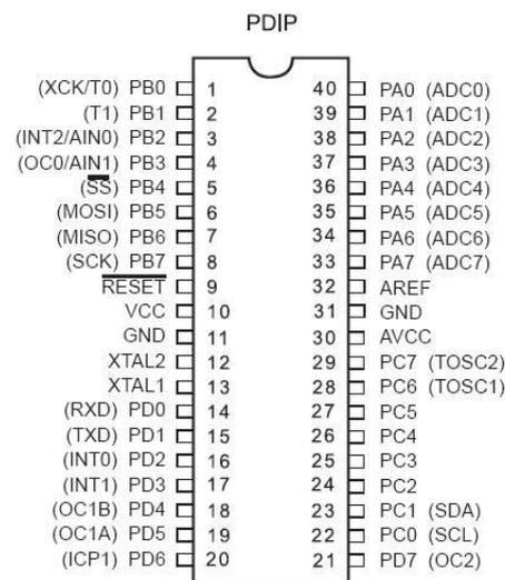
Figure 1. Atmega 8535 Pin Configuration [10, 11]
