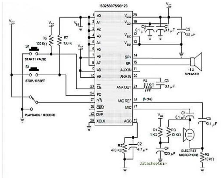
Figure 7. ISD25120 sound recorder IC
