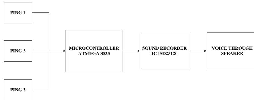
Figure 5. Block diagram of the system tool design
