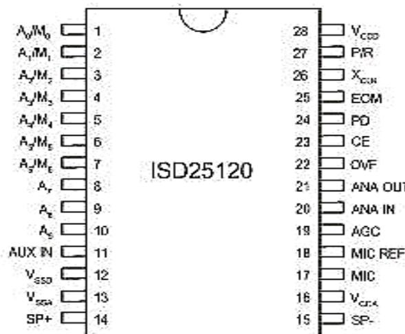
Figure 4. ISD25120 device pinouts
