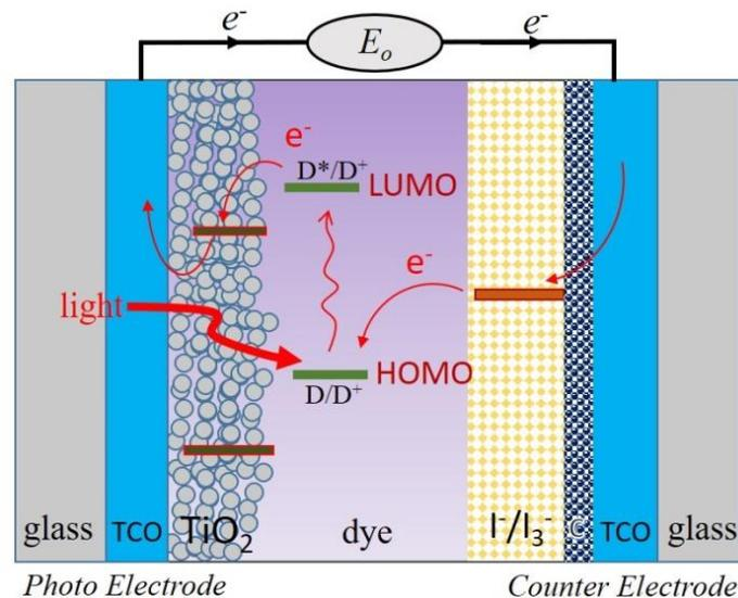
Figure 1. DSSC basic principle for sensor application
