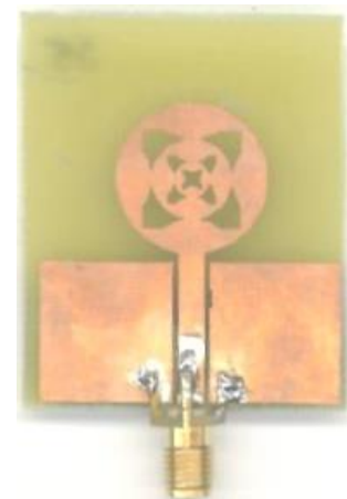
Figure 3. The fabricated fractal CPW antenna
