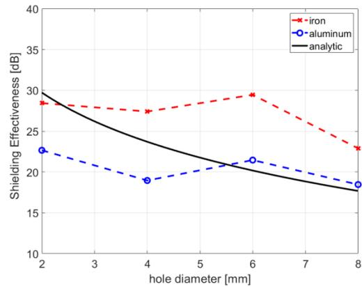
Figure 4. Shielding effectiveness of holey iron and aluminum sheets
