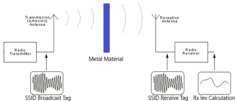
Figure 1. Measurement Method
