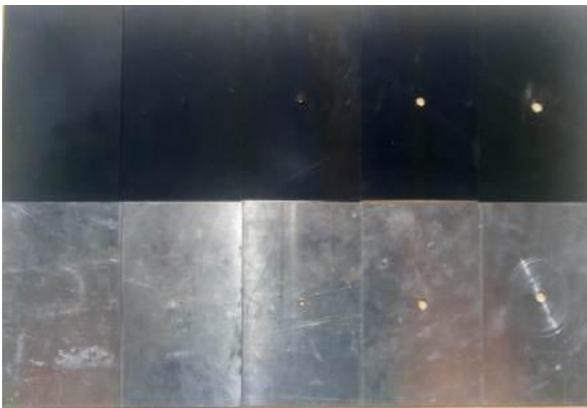
Figure 3. Aluminum & iron metal sheet specimens, from left to right (hole with a diameter of 2 mm, 4 mm, 6 mm and 8 mm)
