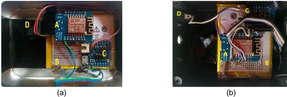
Figure 2. (a) Transmitter and (b) receiver circuitry
