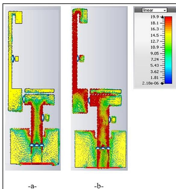
Figure 10. Current distribution of the proposed antenna: (a) ON state at 2.45 GHz resonant freq., (b) OFF state at 5.4 GHz resonant freq.
