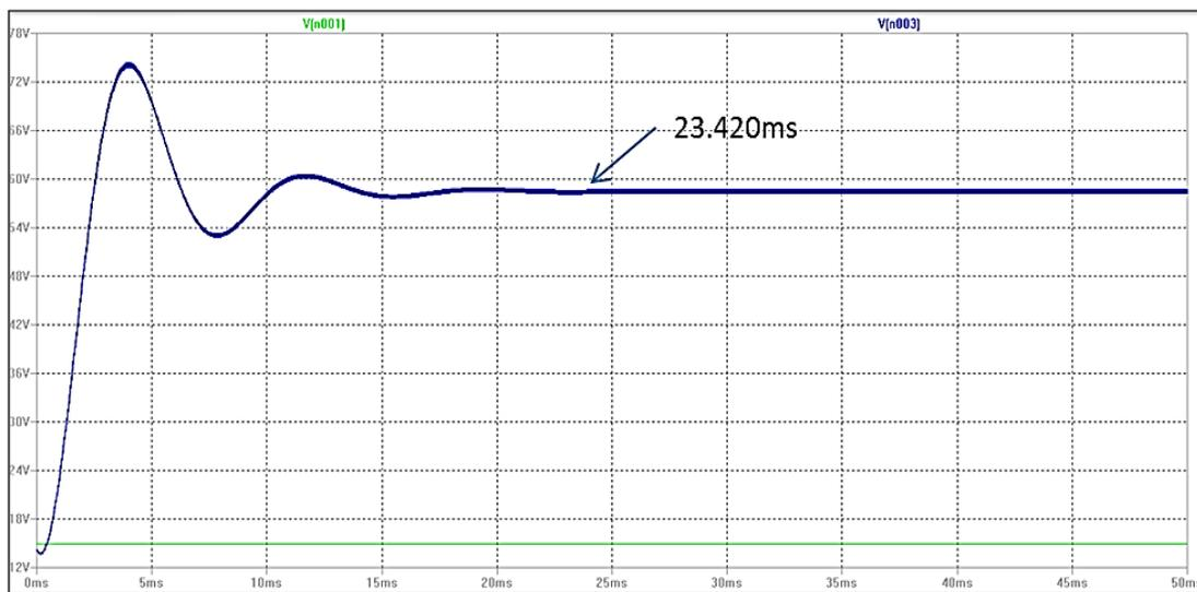
Figure 4. Output voltage across the load resistor R4
