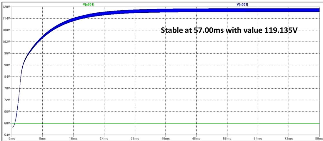
Figure 15. Output voltage at R2 and C4
