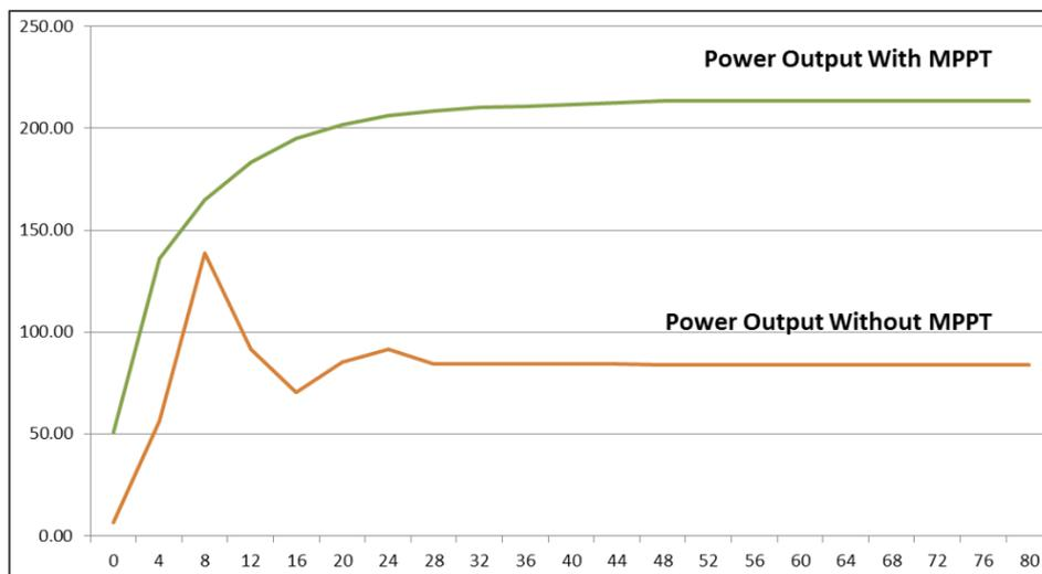
Figure 18. Output power with and without MPPT
