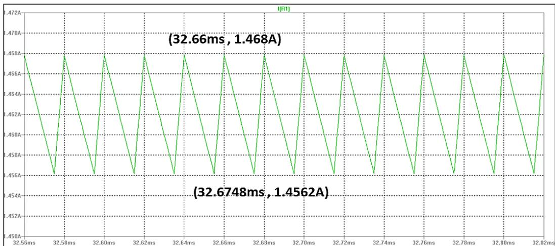
Figure 7. The average current flowing through R4
