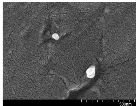
Figure 5. FESEM micrographs for the LDPE-5 sample
