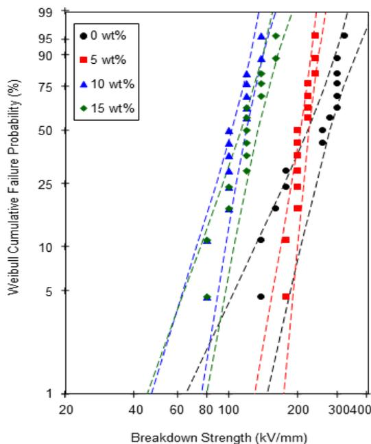
Figure 1. Weibull distribution analysis of DC breakdown strength
