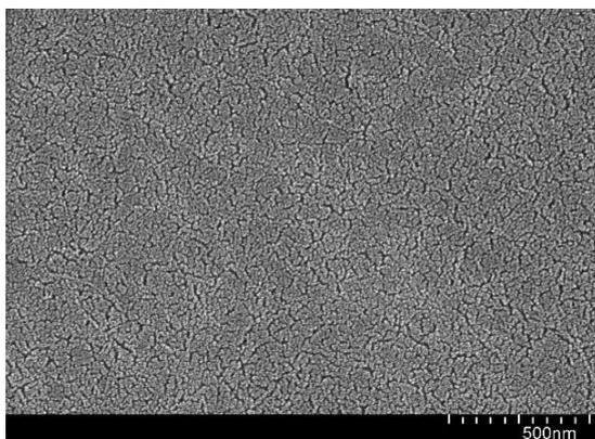
Figure 4. FESEM micrograph for the unfilled LDPE sample/
