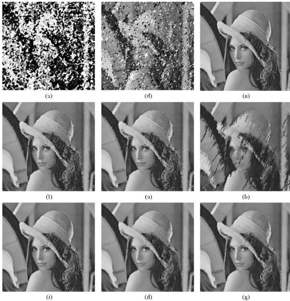
Figure 3. The filtering results of Lena image corrupted by 80% salt and pepper noise; (a) free-noise image, (b) MF, (c) DWMF, (d) BPDF, (e) SMF, (f) AMF, (g) NAFSM, (h) MDBUTMF, (i) DAMF
