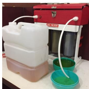
Figure 1. The equipment used for oil filtration
