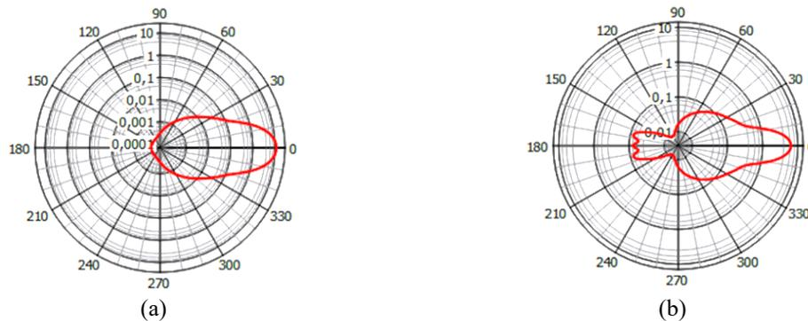
Figure 1. Angular scattering amplitudes of pc-LEDs adding  $\text{CaCO}_3$  (a) and  $\text{TiO}_2$  (b)
