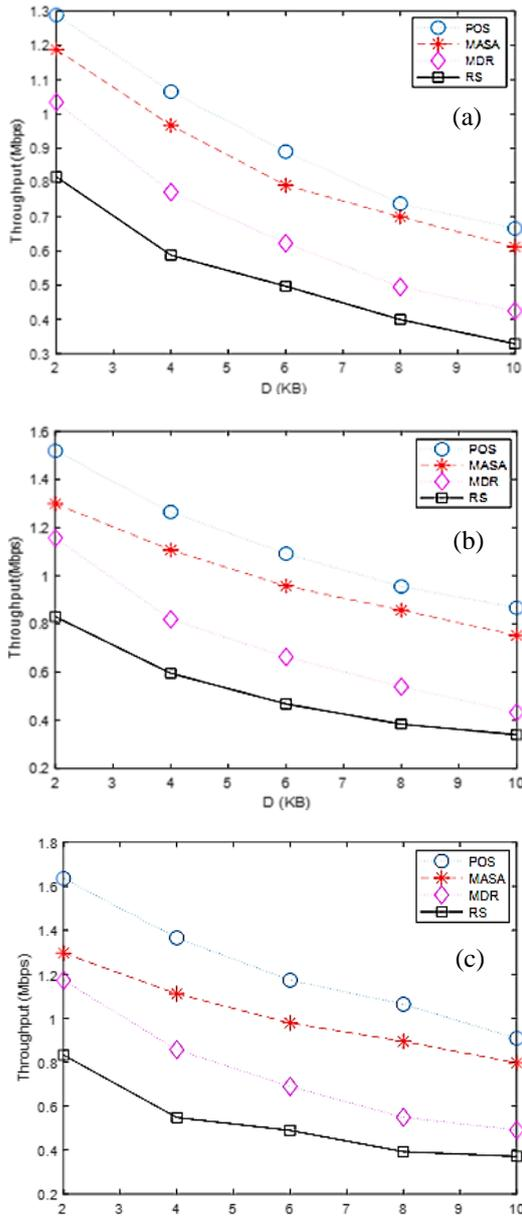
Figure 6. Throughput vs data packet size:
