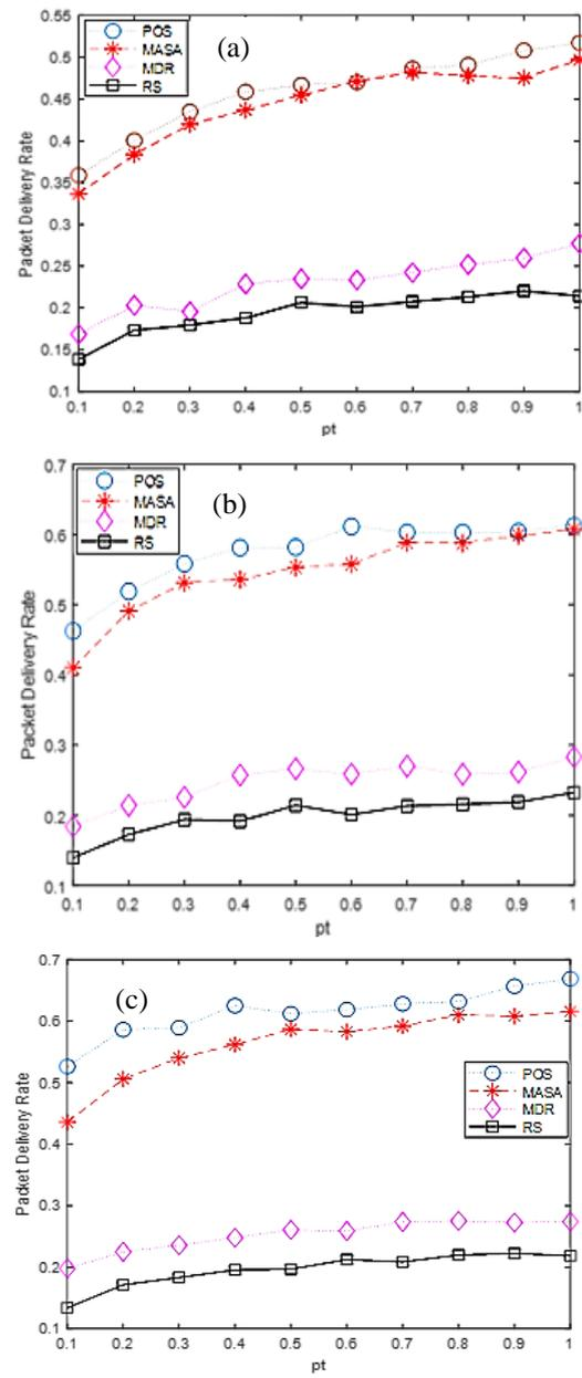
Figure 11. PDR vs transmission power: (a) PI = 0.3, (b) PI = 0.6, (c) PI = 0.9
