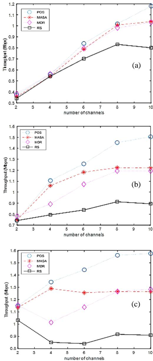
Figure 8. Throughput vs number of channels: (a)  $P_I = 0.3$ , (b)  $P_I = 0.6$ , (c)  $P_I = 0.9$
