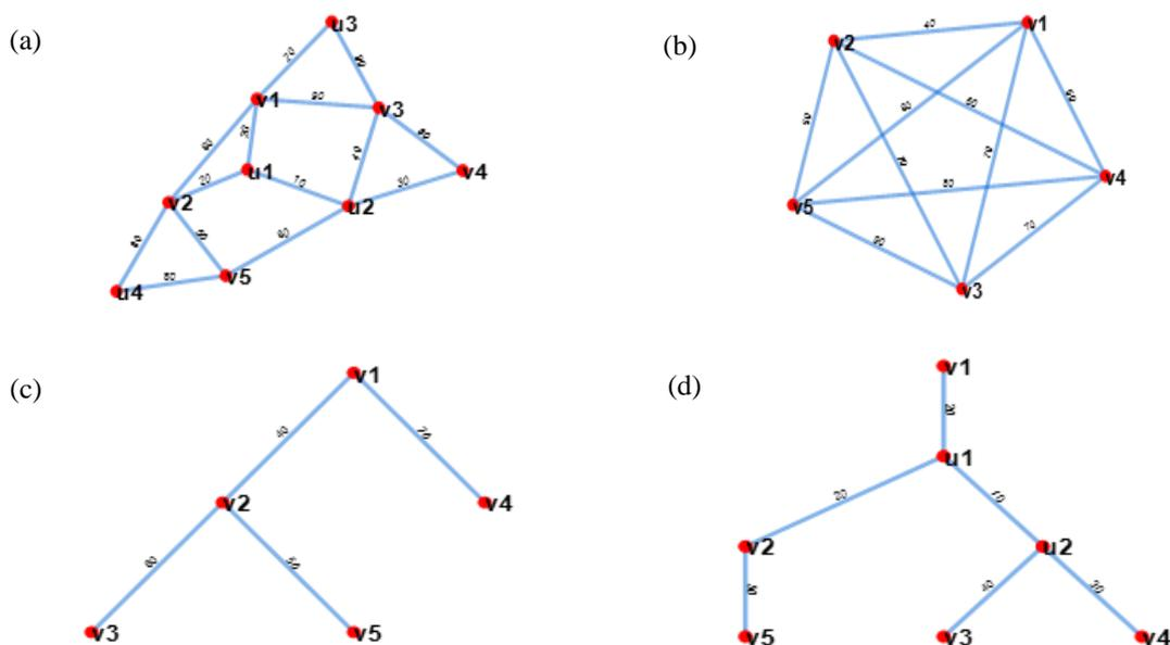
Figure 2. Steiner minimal tree algorithm: (a) undirected graph  $G$ , (b) the metric closure  $G_L$ , (c) the  $MST T_L$ , (d) the SMT  $T$
