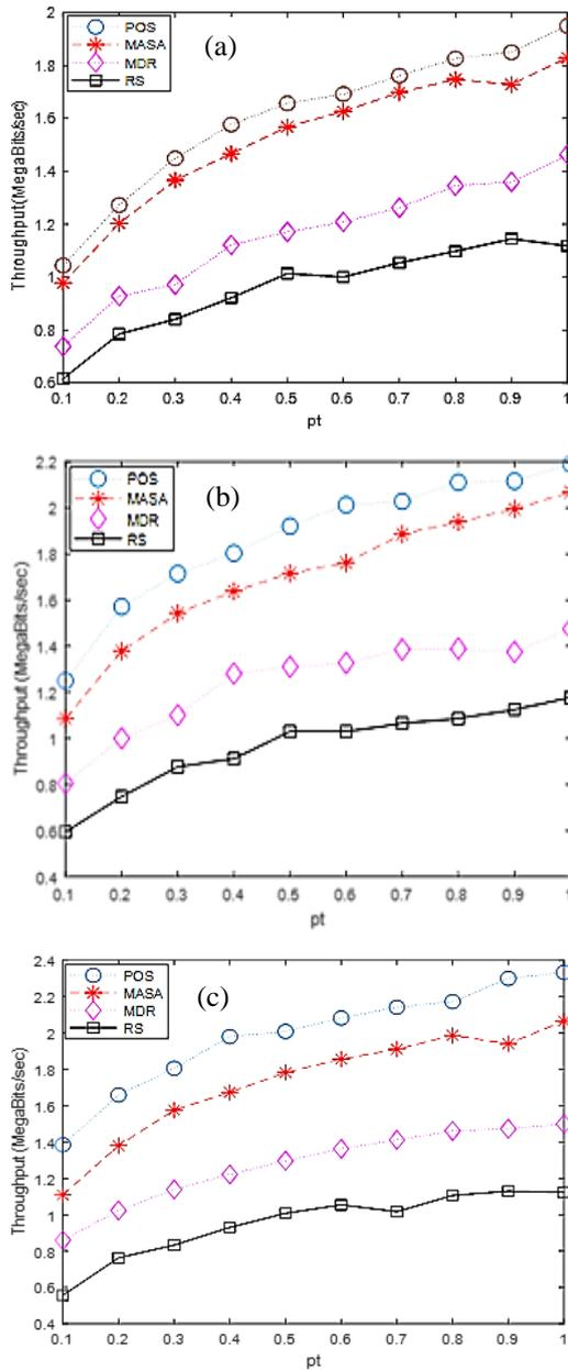
Figure 10. Throughput vs transmission power: (a) PI = 0.3, (b) PI = 0.6, (c) PI = 0.9
