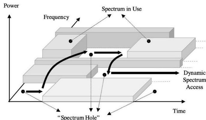
Figure 1. Spectrum for PU and SU in the network
