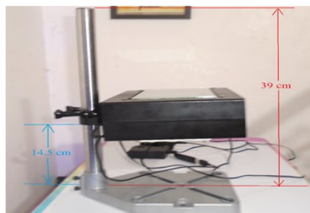
Figure 7. The prototype with the height adjustment set-up
