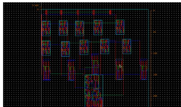
Figure 8. Layout of VCO quantizer
