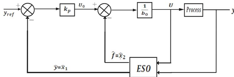
Figure 3. ADRC structure of a first order system
