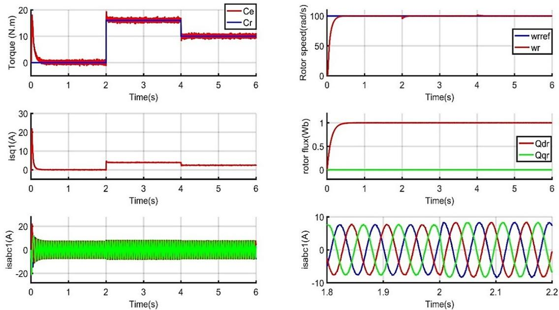
Figure 6. Operation of the DSIM controlled by ADRC regulators with load variation
