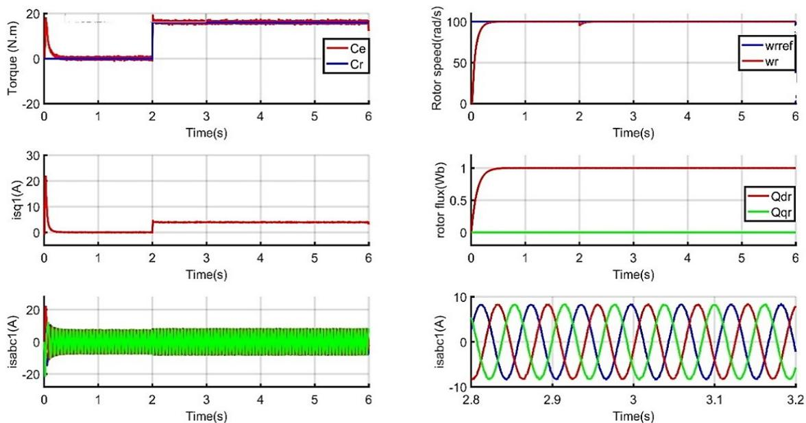
Figure 8. Operation of the DSIM with rotor resistor variation, the moment of inertia variation and the stator inductances variations ( $R_r = 2 \cdot R_{rn}$ ,  $J = 2 \cdot J_n$  and  $L_{s1,2} = 2 \cdot L_{s1,2}$ ) at  $t=3$  s
