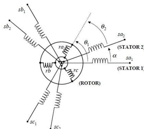
Figure 1. DSIM windings
