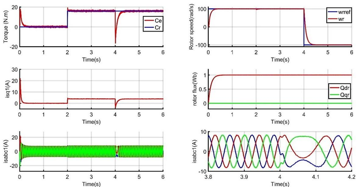
Figure 7. Operation of the DSIM with inversion speed
