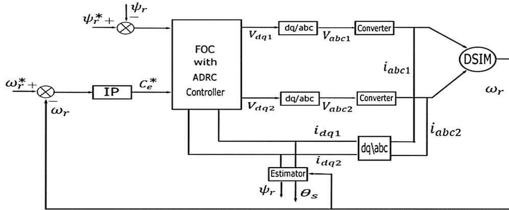
Figure 4. Direct field-oriented control of the DSIM
