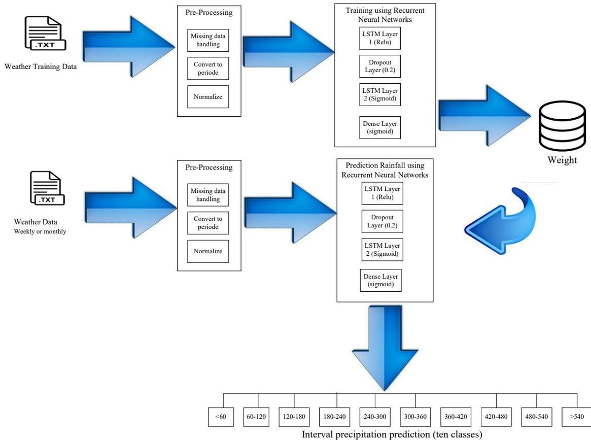
Figure 1. Precipitation prediction model
