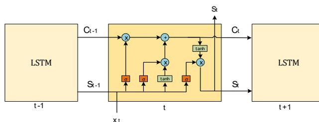
Figure 3. LSTM architecture
