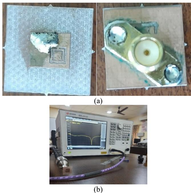
Figure 8. Realized antenna and measurement setup;
