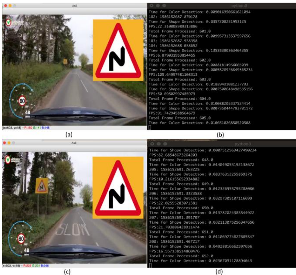
Figure 6. (a, c) TSD with pre-processing system, (b, d) Number of frames processed and the time processing
