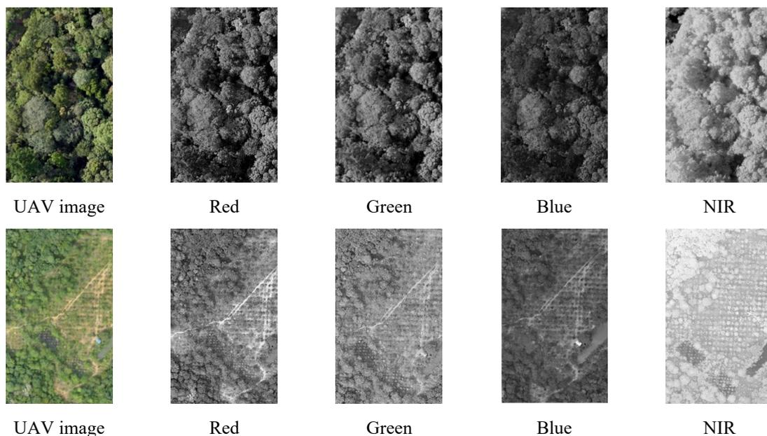
Figure 2. Comparison of UAV visual images with its each respective band
