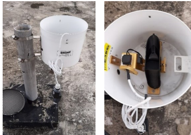
Figure 3. ONSET HOBO RG3-M tipping-bucket rain gauge
