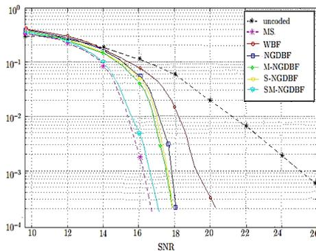
Figure 4. The performance of the  $1/3$  LDPC codes with different decoders over PLC channel in best case
