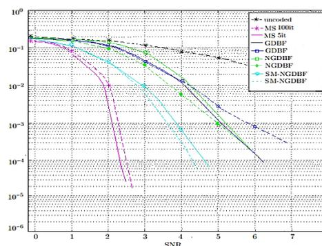
Figure 7. Comparative performance of GDBF, NGDBF, M-NGDBF, S-NGDBF and SM-NGDBF with traditional Min-Sum (MS) with 5 and 100 iterations, WBF algorithms
