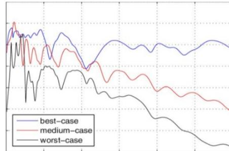
Figure 3. Amplitude responses of the indoor PLC channel scenarios
