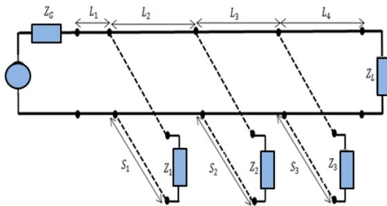
Figure 2. Simplified structure of PLC network used in bottom-up channel modeling
