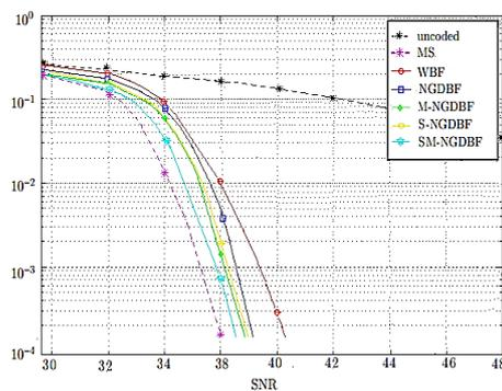
Figure 6. The performance of the  $1/3$  LDPC codes with different decoders over PLC channel in worst case
