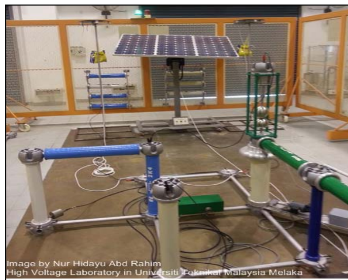
Figure 1. Impulse voltage generator configuration in high voltage laboratory to produce high voltage
