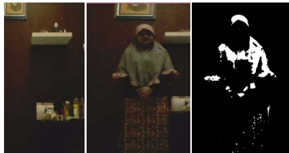
Figure 1. Left: the reference frame, Middle: the current frame, Right: the detected motion [5]
