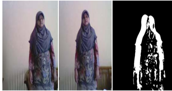
Figure 2. Left: the previous Frame, Middle: the current frame, Right: the detected motion
