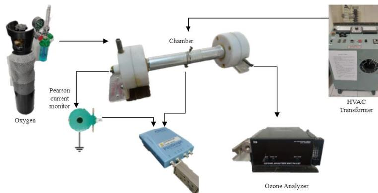
Figure 3. Experimental setup
