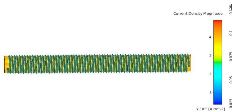
Figure 6. Distribution of current density on the screw model
