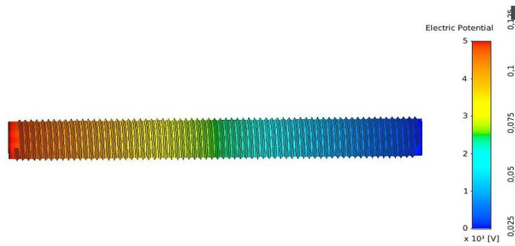
Figure 4. Electric potential distribution on the screw model
