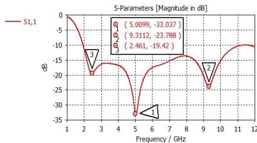
Figure 3. Return loss s-parameters of antenna monopole
