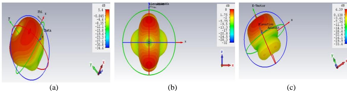
Figure 6. 3D radiation pattern gains of monopole antenna; (a) at 2.4GHz, (b) at 5GHz, and (c) at 9.3GHz
