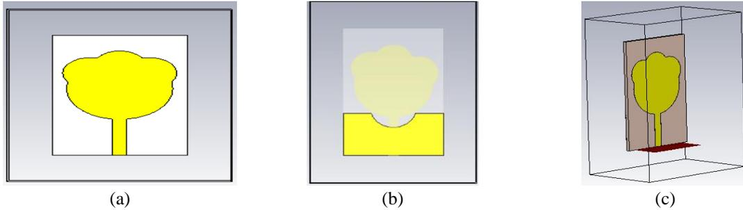
Figure 1. The geometry of monopole antenna; (a) front part, (b) back part, and (c) side part
