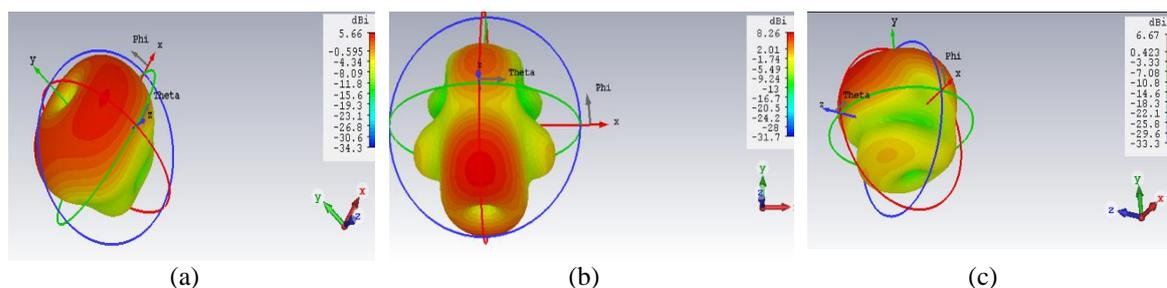
Figure 8. 3D radiation pattern directivity of monopole antenna; (a) at 2.4GHz, (b) at 5GHz, and (c) at 9.3GHz
