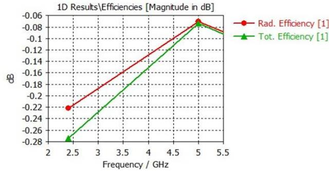
Figure 2. The radiation efficiency of the suggested antenna at 5 GHz
