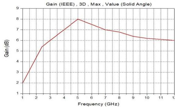
Figure 7. The curve of antenna gain
