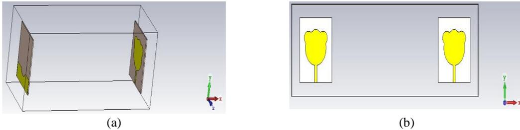
Figure 9. Design antenna structure; (a) face to face and (b) side by side
