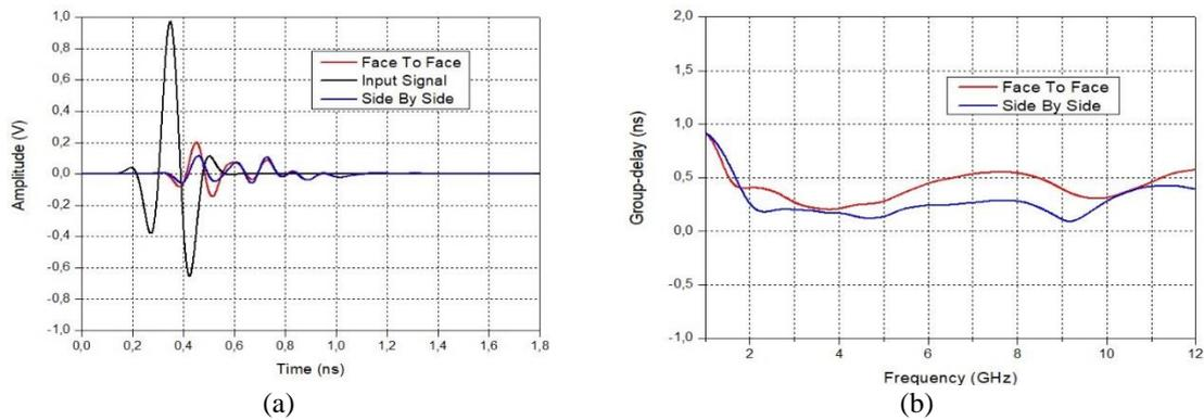
Figure 10. Simulated; (a) simulated time domain analysis (input and output signal) and (b) the simulated group delay of the proposed antenna
