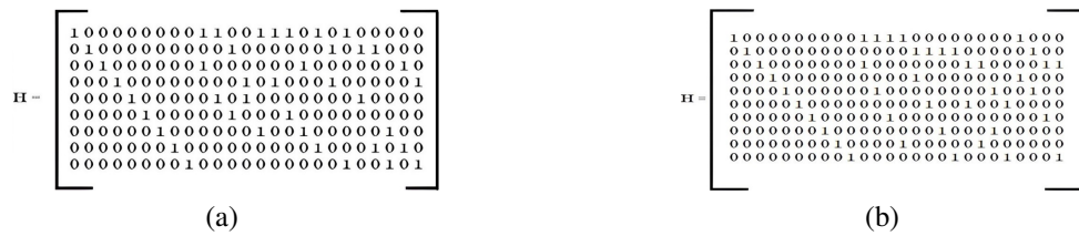
Figure 4. Optimized H-matrix for error correction; (a) 6-bit adjacent error and (b) 7-bit adjacent error
