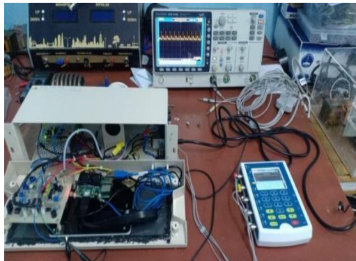
Figure 4. ECG data collection using an ECG simulator which is then used for offline EDR analysis
