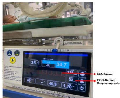
Figure 7. The ECG signal and respiratory rate value are displayed on the baby incubator monitor display
