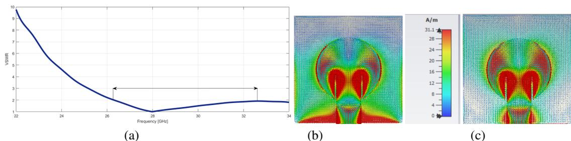
Figure 4. VSWR and surface currents; (a) the graph depicting the VSWR concerning frequency corresponds to the proposed antenna's operation, (b) proposed antenna's current distribution at 28 GHz, and (c) conventional antennas current distribution at 28 GHz
