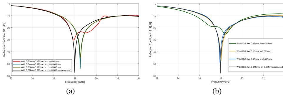
Figure 3. Comparison of antenna performance concerning the combination of different shapes of DGS; (a) bandwidth and reflection coefficient concerning DGS 'a' and (b) bandwidth and reflection coefficient concerning DGS 'a' and 'Ax'
