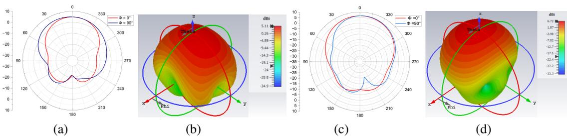
Figure 6. Radiation patterns for the proposed antenna with DGS and without DGS operating at 28 GHz; (a) E-plan and H-plan without DGS, (b) 3D radiation pattern without DGS, (c) E-plan and H-plan with DGS, and (d) 3D radiation pattern with DGS
