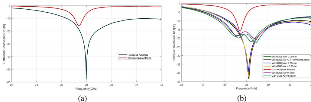
Figure 2. Comparison of antenna performance between conventional and proposed antenna; (a) bandwidth and reflection coefficient concerning 'a' and (b) bandwidth and reflection coefficient concerning  $A_x$
