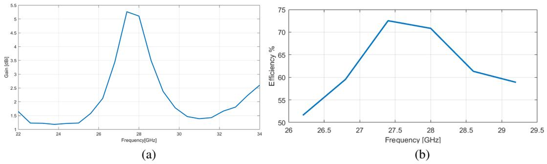
Figure 5. The graph depicting the antenna gain and efficiency concerning frequency for the proposed antenna; (a) gain and (b) efficiency
