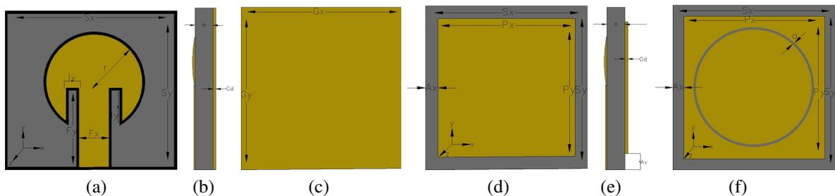
Figure 1. Conventional circular patch antenna design: (a) front View, (b) side view, (c) back view. Proposed antenna with DGS of: (d) back view with first step (e) side view, and (f) back view with second step of DGS
