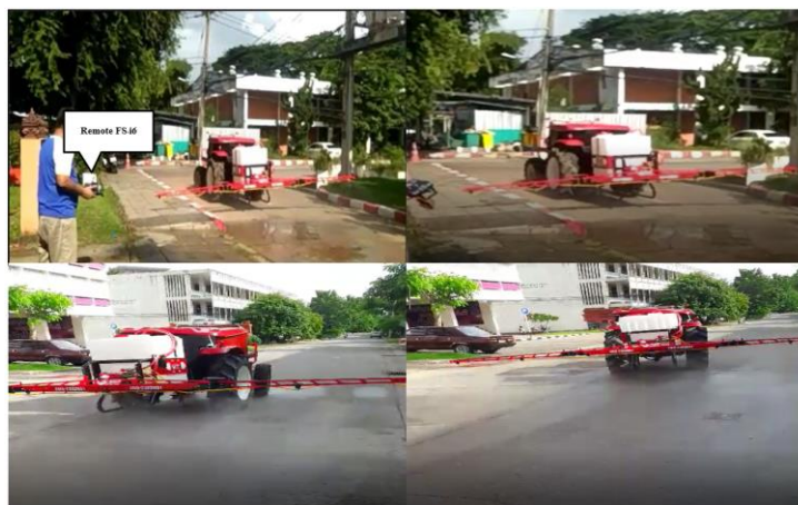
Figure 15. Testing drive of an agricultural tractor using radio remote control on the road
