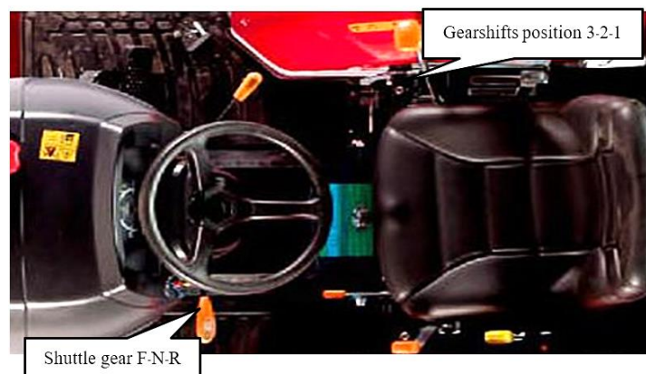
Figure 1. The three-position gear selector lever stalk of the prototype tractor
