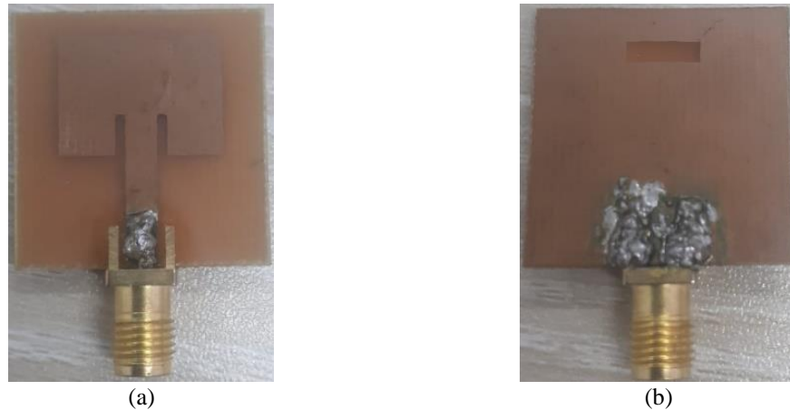
Figure 6. Proposed antenna with rectangular DGS patterns constructed on a FR4 PCB; (a) front side and (b) back side
