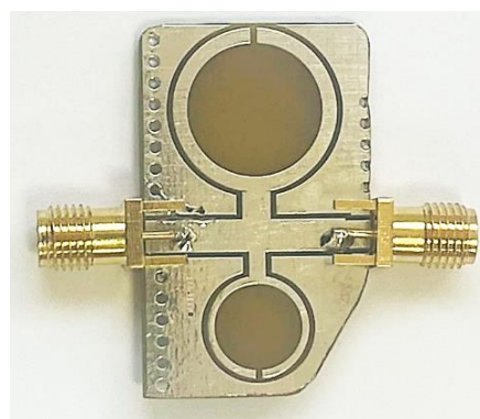
Figure 3. Image of the manufactured prototype of the proposed zero-order resonator
