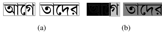
Figure 4. An example of word segmentation by the filled rectangle: (a) connected component: the two words are segmented into three connected components. Those components are shown inside the rectangles and (b) extended and filled the horizontal length of the rectangle covering the word is extended and filled. Therefore the sub-section of the words are merged and separated as a single word
