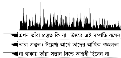
Figure 2. The histogram in the vertical and horizontal orientations shows the count of black pixels for each direction respectively. The dotted lines indicate the separation between the lines of text
