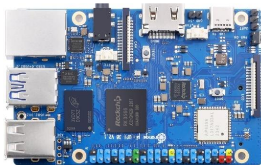
Figure 1. Orange Pi 3B with Rockchip NPU RK3566
