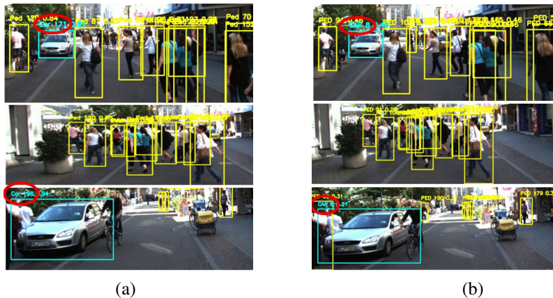
Figure 10. Track results: (a) decoupled DeepSORT based on Kalman filter and (b) decoupled DeepSORT based on \alpha\beta filter
