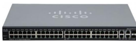
Figure 4. A Cisco switch
