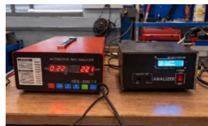
Figure 6. Standard emission test equipment and design tools
