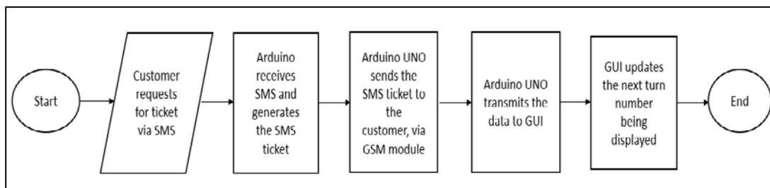
Figure 3. The System Operational Flow Chart for Requesting SMS Ticket Remotely Via SMS
