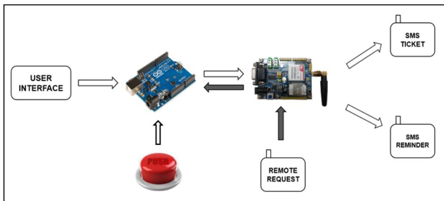
Figure 1. Architecture of Queue Management System
