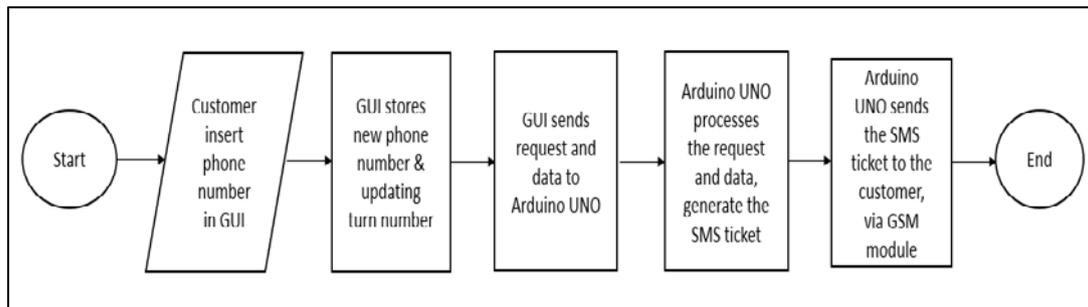
Figure 2. The System Operational Flow Chart for Requesting SMS Ticket Using GUI
