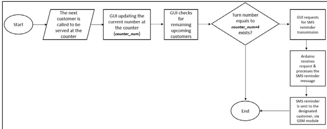
Figure 4. The Flow Chart of SMS Reminder Generation and Transmission
